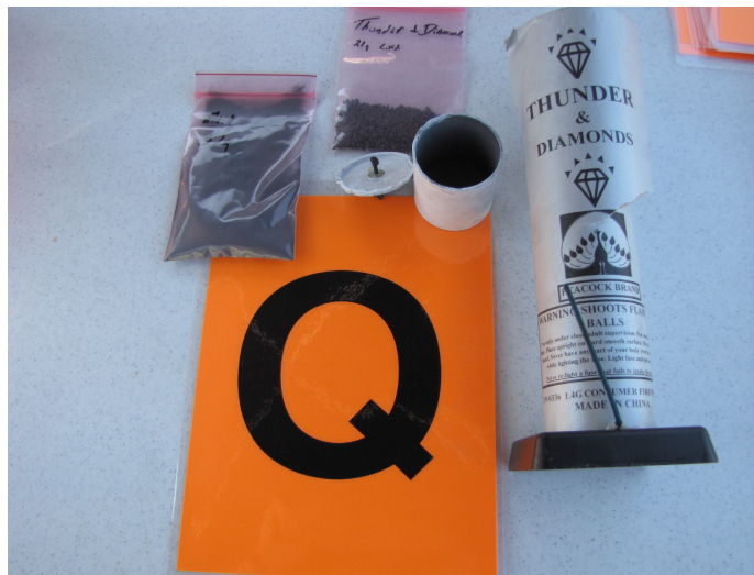
Disassembled “Thunder & Diamonds” tube, showing components including hard plastic projectile shell (at top right corner of orange card)
